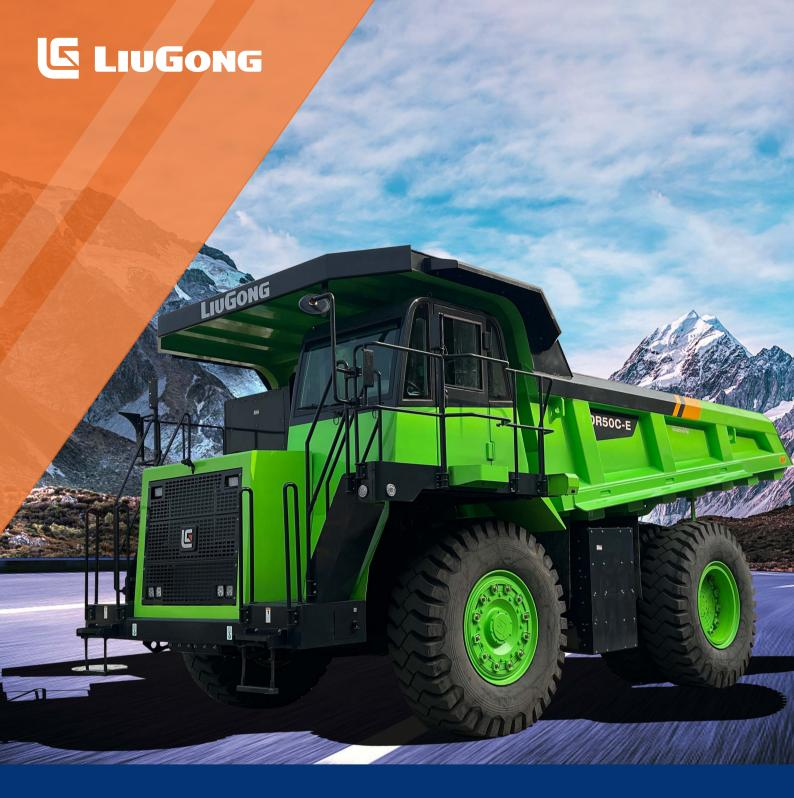
**Max. Gross Machine Weight** 85,000 kg **Net Machine Weight** 40,000 kg **Payload** 45,000 kg **Engine** HL13200 480 kW (644 hp / 653 ps) @ 1,050 rpm **Rated Power Max. Speed** 55 km/h **Reverse Speed** 10 km/h **Struck Capacity** 22 m<sup>3</sup> **Heaped Capacity (SAE 2:1)** 30 m<sup>3</sup>
